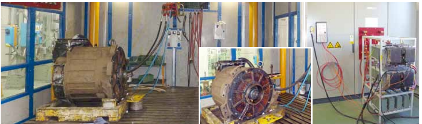
Asynchronous traction motor test bench
